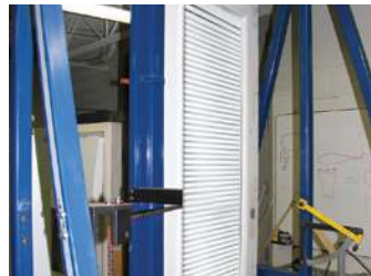
50,000 slam cycle test
