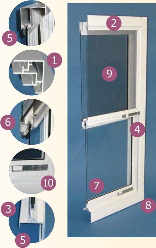
1. High tempered 6063 T-6 aluminum coupled with chambered frame design - provide unparalleled rigidity, ensuring ease of installation and long term durability.
